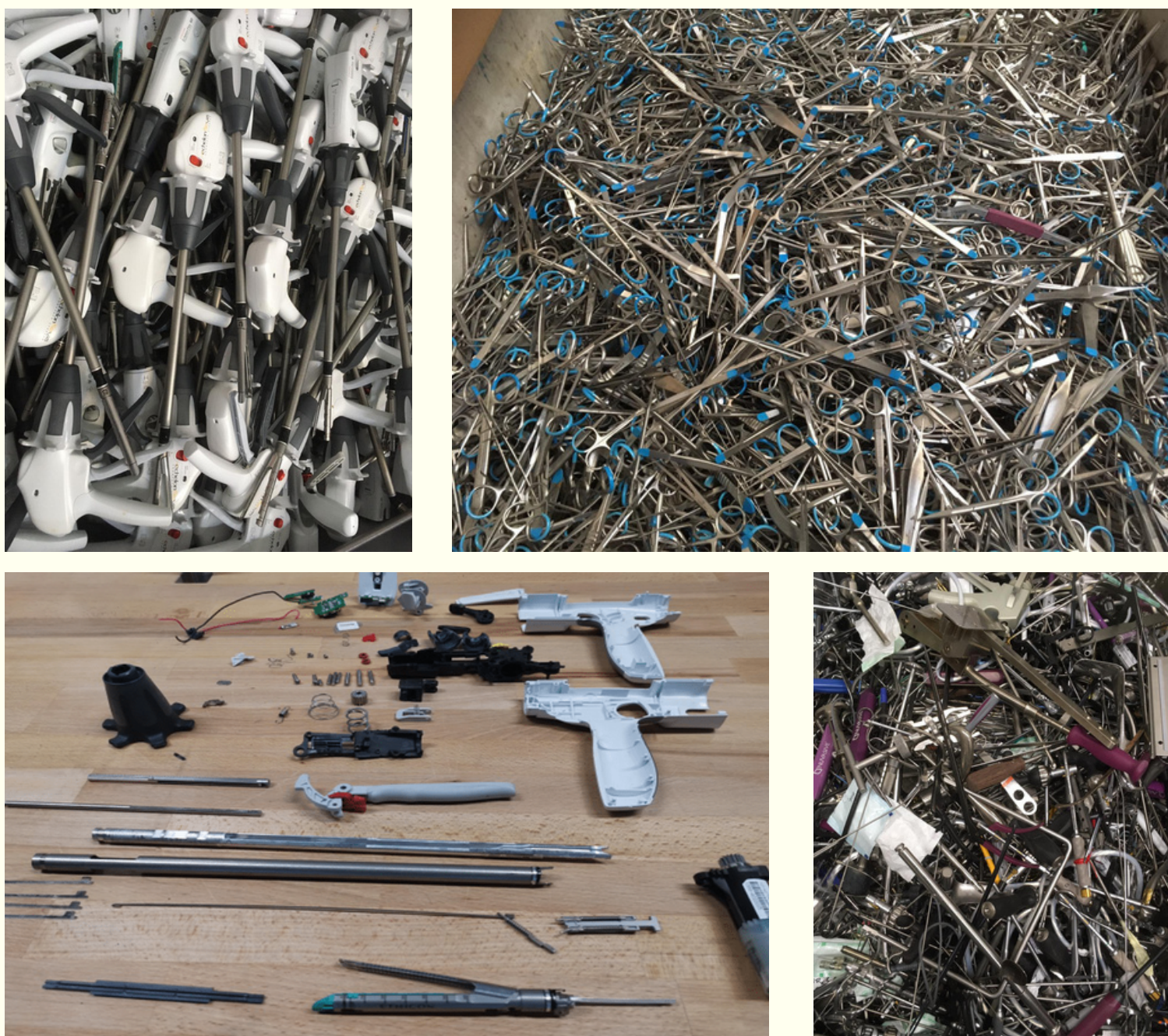
F.L.T.R. Top: Discarded surgical staplers, discarded surgical scissors. F.L.T.R. Bottom: Disassembled surgical stapler, Other disposable equipment.
