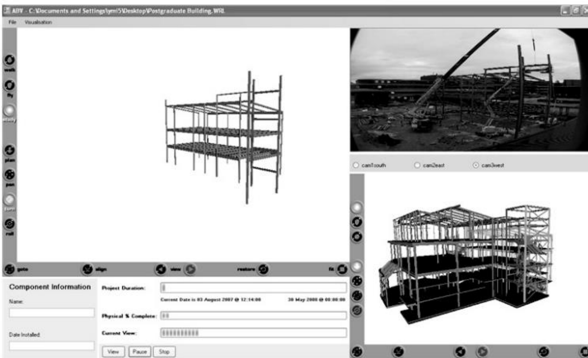
Figure 40 - Videogrammetry 3D model compared to original 3D model (source (Ibrahim, Y. M., Kaka, A. P., Aouad, G., Kagioglou, M., 2008) )
